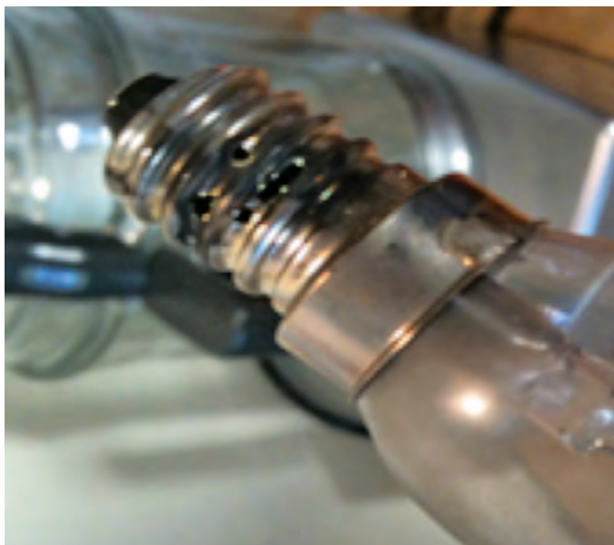
Light bulbs should make a complete connection with the socket
