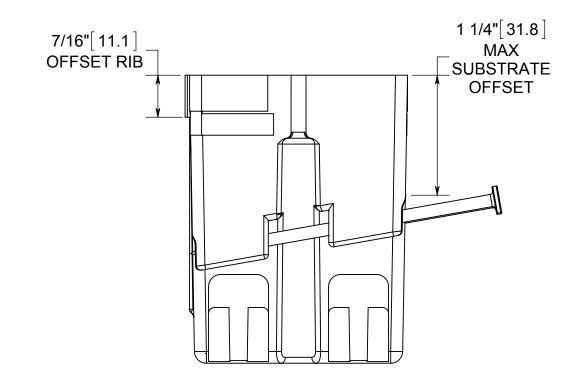
NOTES: 1.) BOX MATERIAL: FIBERGLASS REINFORCED POLYESTER, NAIL MATERIAL: PLATED CARBON STEEL 2.) UL LISTED WITH 2 HOUR FIRE RATING FOR WALL AND CEILING
