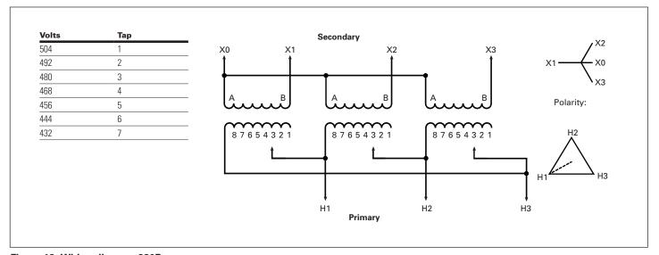
Figure 12. Wiring diagram 280B
