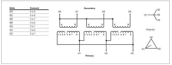
Figure 11. Wiring diagram 275A
