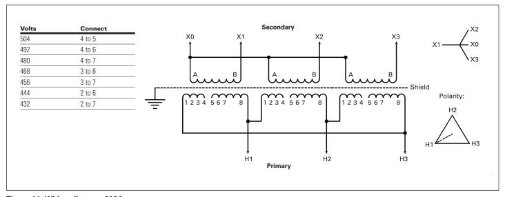
Figure 14. Wiring diagram 292A
