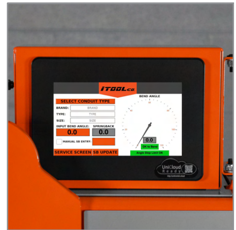
Touch Screen Allows User to Pre-Save Springback Values for up to 5 Brands
