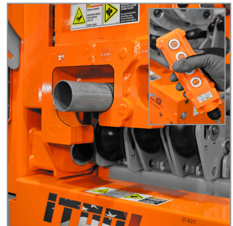
Hydraulic Load Bar Locks Conduit In Place with the Push of a Button
