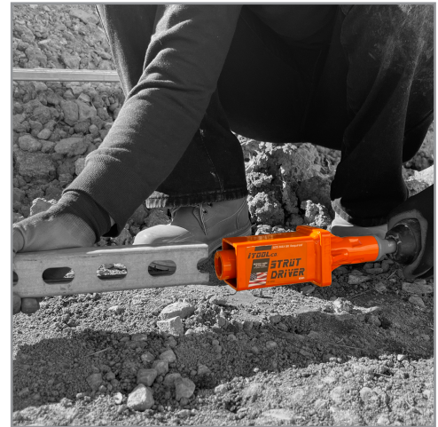
End Receiver Accepts 1-5/8" Strut
