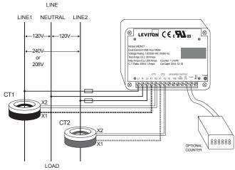
Leviton recommends solid core transformers (CTs) for revenue-grade accuracy. Our 100A and 200A color coded CTs assist with correct installation by indicating phase monitored. Split core CTs are also available upon request for applications where power cannot be interrupted during installation. Our 100-200 Amp Split Core CTs offer +/-1.0% accuracy.
