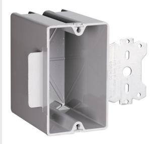
Single Gang, Deep Bracket Box for Wood and Steel Studs with Quick/Click Entries. 3/8" offset for wood and steel stud mounting. For use with 3/8" to 5/8" wallboard. 100 pack.
