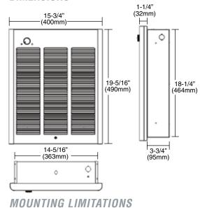
Do not install heater closer than 8" from floor or adjacent wall surface, behind towel rack or door, upside down or side up, in floor, ceiling or closet.
