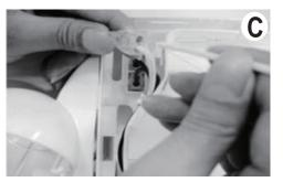
3. In upper left corner of housing wire channel connect input leads using push nuts and jumper wire provided to route wires to j-box. Connect battery after AC power can be continuously provided to exit and snap face plate onto housing. Remote lamp option: Connect remote lamps to yellow and blue wires using push nuts and jumper wire provided to route wires to j-box.
