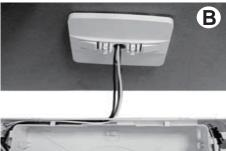
2. Fasten canopy to j-box bracket. Remove face plate from housing. Remove hole plug and dress leads through housing wire channel. Snap exit housing onto canopy.
