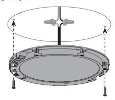
4. Install surface cover to light body. Ensure lock marks are aligned.
