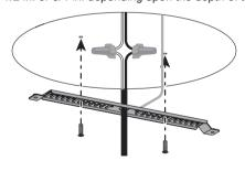
a. Push light body up to bracket. Be sure to align the sensor towards the door or entry point.
