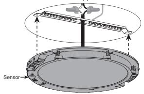
**b.** Rotate light body clockwise to engage with the bracket.
