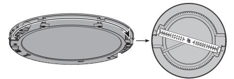
**6.** Once the light body is in place install the two 1/2 in. screws to secure light body to the bracket.
