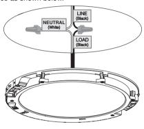
3. Install the light body with two screws.
