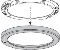
4. Tighten bracket until flush against the ceiling surface. DO NOT over tighten. Over tightening will bend the bracket and make installation of lamp difficult.
