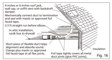
The ducting from this fan to the outside of the building has a strong effect on the air flow, noise and energy use of the fan. Use the shortest, straightest duct routing possible for best performance, and avoid installing the fan with smaller ducts than recommended. Insulation around the ducts can reduce energy loss and inhibit mold growth. Fans installed with existing ducts may not achieve their rated air flow.
