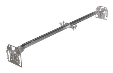
The nVent CADDY 512SA T-Grid Box Hanger is designed to answer the challenge of accommodating multiple electrical box depths and acoustical tile reveal options in industrial ceilings. The 512SA easily snaps into place, with tool-free installation saving time and increasing efficiency on the jobsite. For added flexibility, the 512SA can be adjusted with the push of a button – an important feature for overhead installation projects.
