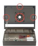
Easy installation options with integral wiring compartment. Mount directly over standard recessed or surfacemount junction boxes or use one of three ½" threaded conduit hubs for surface conduit mounting.
